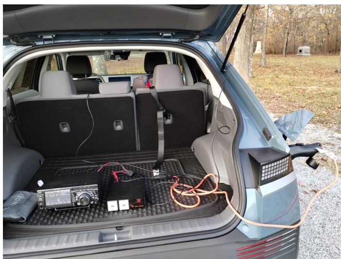
NN4NT operation at Chickamauga National Military Park (US-0716) using an FTDX-10 and a 15m hamstick
