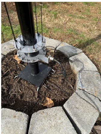
W1WSF fabricated a custom steel tilting base that included radial attachment points.
