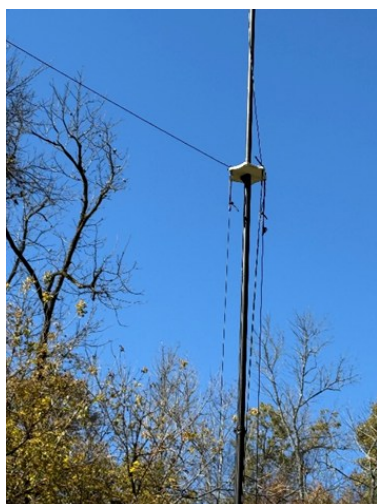
W1WSF's Inverted L antenna on his DX Commander Signature 9 mast
