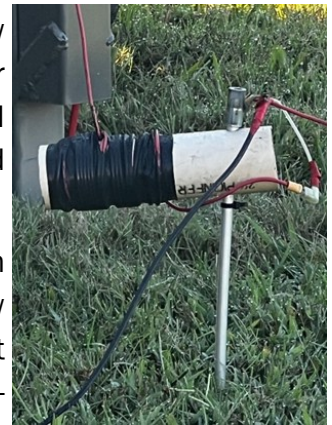
Picture 9: Connection to inverted-L element
