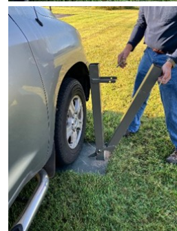
Pictures 2 & 3: Tilt-over antenna raising fixture
