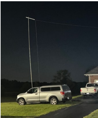
Picture 8: Inverted-L antenna
