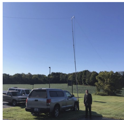
Picture 7: The dipole antenna at ~40 feet
