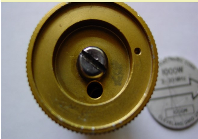
Figure 3: Bird slug with aluminum face plate and excess glue removed.
