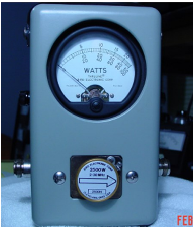
Figure 1: My Bird Model 43 with a 2.5KW plug-in element that covers 2-to-30 Mhz.
