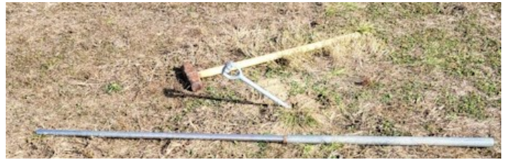
Above: The three anchors were successfully screwed into hard, rocky soil.
