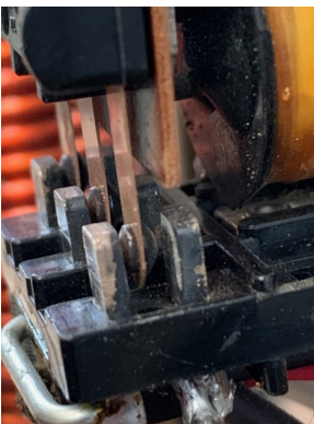
AG4W cleaned the I/O relay contacts while he was inside the amp.
