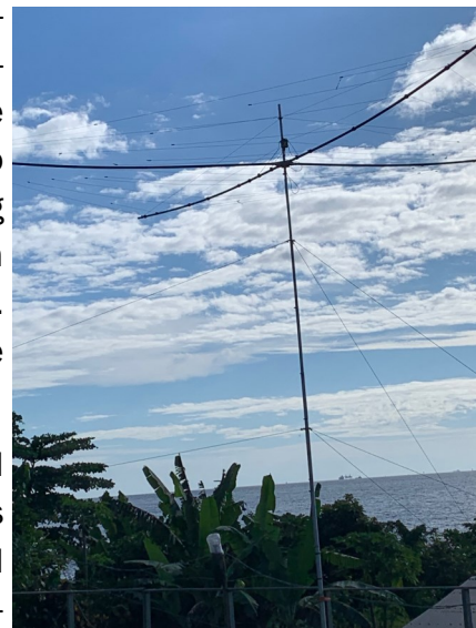
Included in TJ9MD's temporary antenna farm are four spiderbeam antennas.
