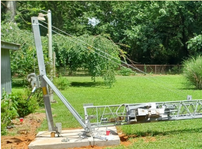
The US Towers winch fixture makes raising and lowering the tower a breeze.
