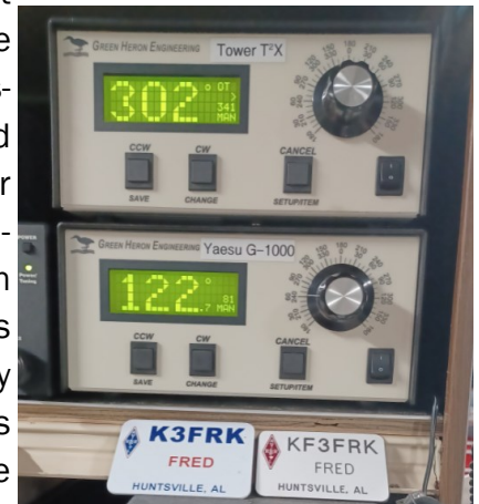
Above: Green Heron Engineering RT-21 Rotator Controllers will allow precise remote control of the rotators
