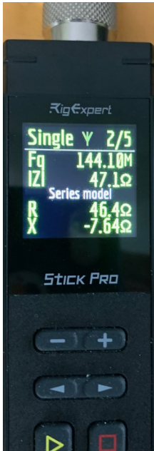
Figure 2 – SWR of AG4W's 2m EME antenna at 144.07 MHz
