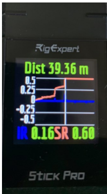
Figure 3 – TDR measurement from AG4W's 80m loop antenna
