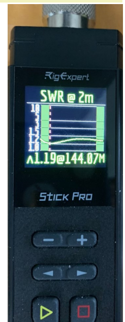
Figure 1 – SWR graph of AG4W’s 2m EME antenna
