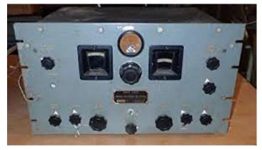
Signal Corps Radio Receiver BC-779-B
