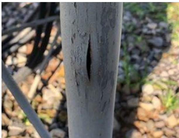
Steel tower leg frozen and busted
