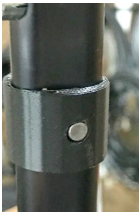
Figure 10. Adapter for 1" ID pipe with dowel pin fully inserted.
