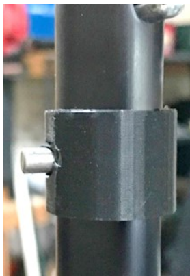
Figure 9. Adapter for 1" ID pipe with dowel pin partially inserted.
