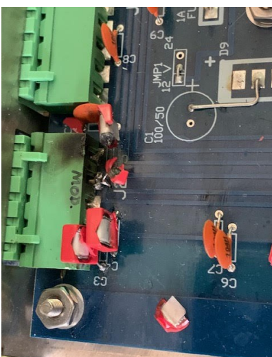
Blown capacitors in AG4W's control box
