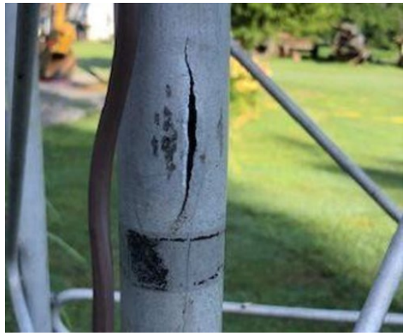
Aluminum tower leg froze and split
