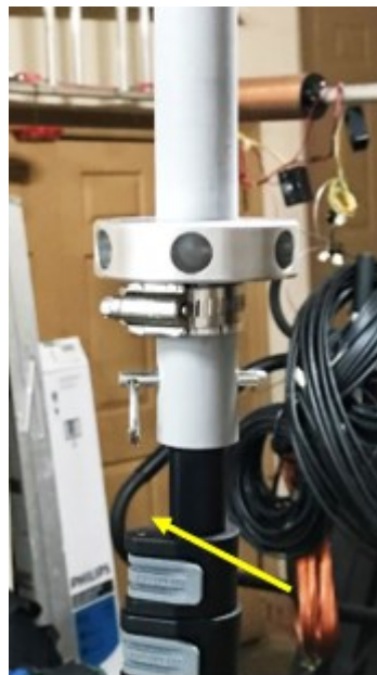
Figure 12. Hex-Beam center column is solidly attached to the mast.
