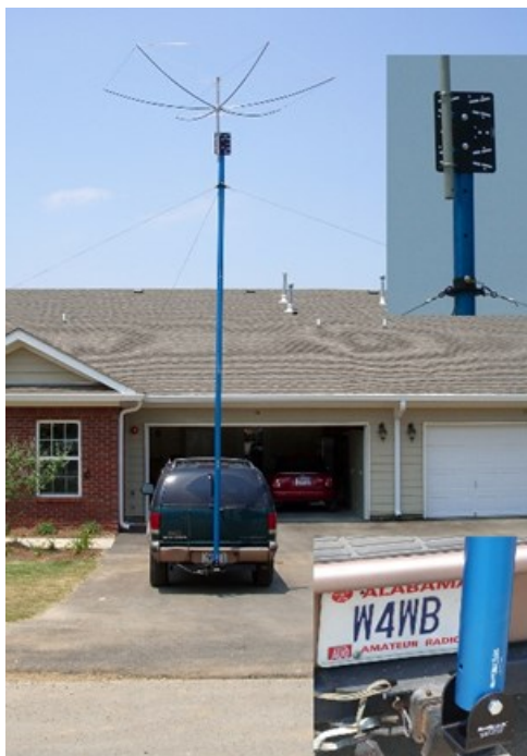
Figure 8. Hex-Beam for 15 m assembled from the Hex-Pac mounted on a Blue Sky Lite mast.
