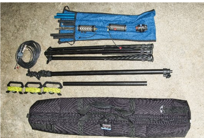
Figure 5. Buddipole Antenna System for 6-40 m and provides tripod with mast and guys.
