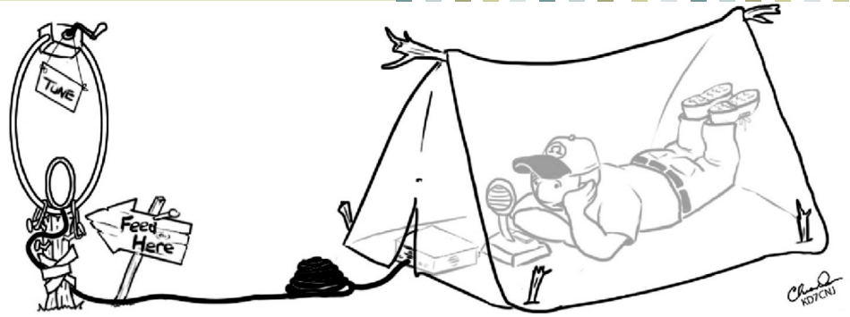
Figure 1—The small gap resonated loop fed by a secondary loop makes a compact portable HF antenna for QRP expeditions. Source: ©2014 Chris Dean, KD7CNU, used with permission.
