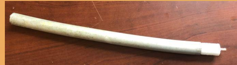
Short Piece of 3/4" 75-Ohm CATV Hardline easy to kink
