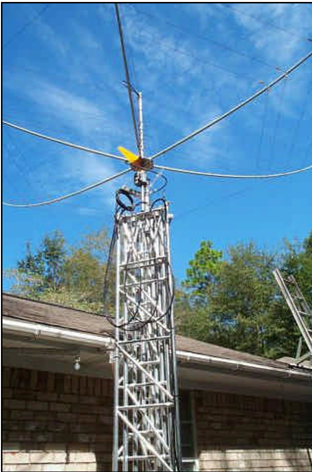
Figure 1. HX-5B Hex-Beam at W2GFF.
