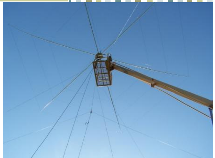
Here's a better view of the hexbeam. The dipole below, later raised to the bottom of the bucket, is oriented for an E-W pattern.
