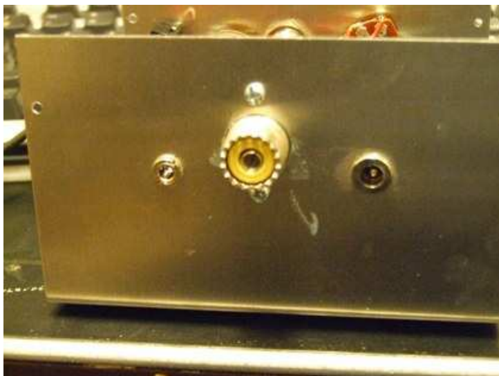
The rear panel, with just enough connectors to get the work done. Audio I/O to the computer is on the left, and power on the right.
