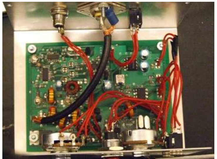
The work gets done here. Note the many surface-mount parts.
