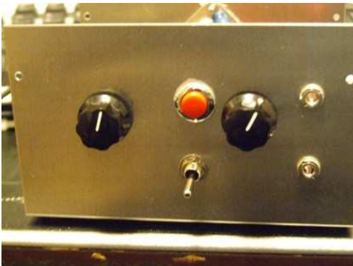
Front Panel—Knobs are for VXO and keyer speed control. The switch is for spotting and the push button for programming the keyer. The jacks are for keyer sidetone and keyer input.
